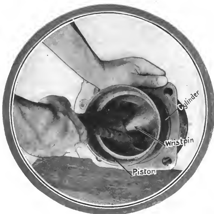
Fig. 3—Method used in an attempt to remove piston from cylinder. This means proved inadequate, as the piston had rusted within the cylinder
